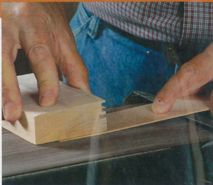
Feather the ends on the inside face. Use a horizontal belt sander. A block spreads pressure and produces a more consistent taper. The taper makes it easier to cut the swallowtails, too.
