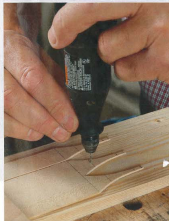
Drill pilot holes. Be sure to hold the drill (a Dremel in this case) perpendicular to the band.
